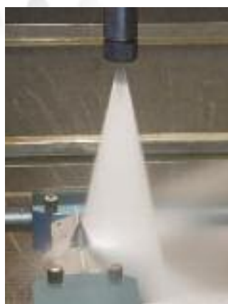
Documentation of a spray impact measurement
