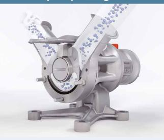
A single sinusoidal rotor creates four evenly sized chambers. As each chamber rotates it gently conveys the fluid from the inlet port to the outlet port. At the same time, the opposite chamber opens to draw in more fluid, resulting in a smooth flow with virtually no pulsation.
