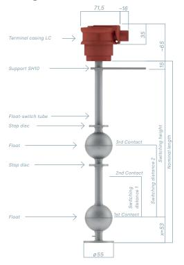
Float switch made of stainless steel with 3 contacts, LC version
