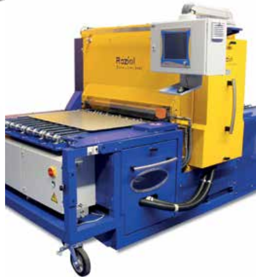
Blank lubricator system with 2 medium circuits
