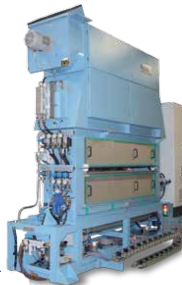
Special lubrication systems for coils, integration in press lines
