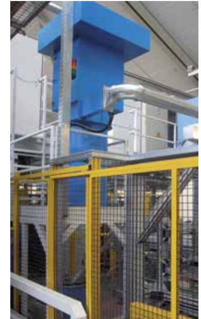
Wet scrubbers for oil mist removal
