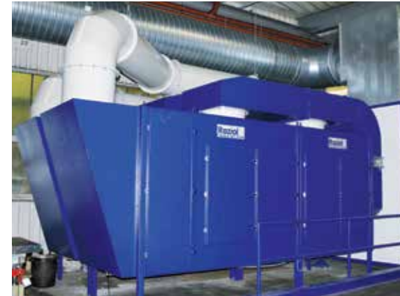
Oil mist cartridge filters for oil mist removal
