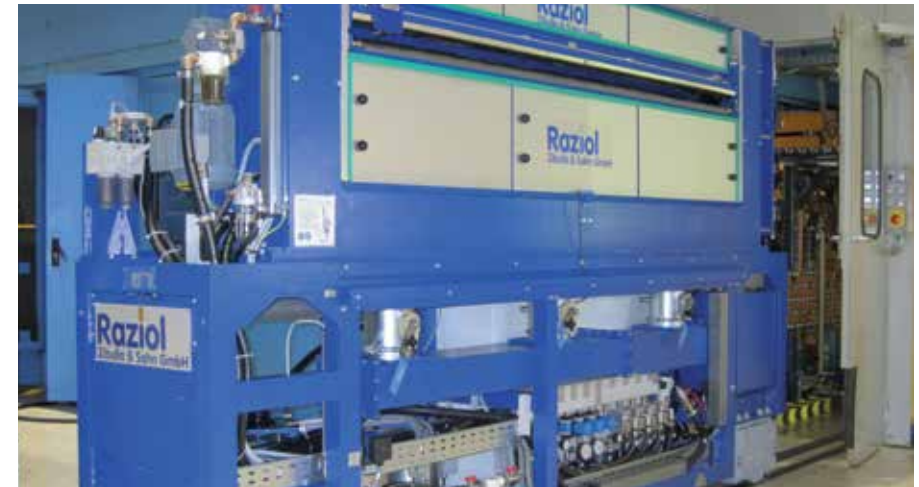
High-performance lubrication system for blanks, can be moved completely out of the line
