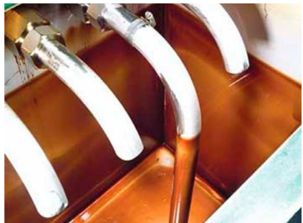
Figure 3. Varnish present in a hydraulic sump. If varnish is detected here, it is almost certainly present in other parts of the system as well. Source: Noria Corporation .
