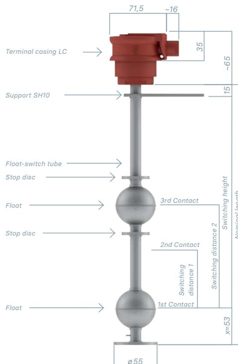
Float switch made of stainless steel with 3 contacts, LC version
