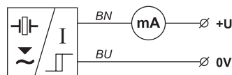
Connection diagram of the ULS sensor with S type output (two-state current switch 4 mA / 20 mA)
