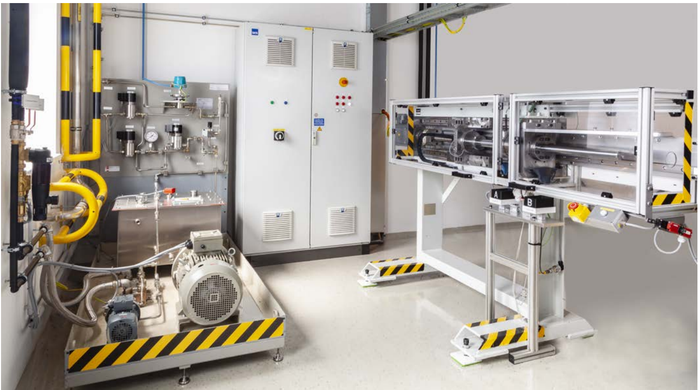
Figure 1. Reciprocating hydraulic seal test rig.
