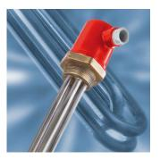
The ETTO screwed rod heater can be used for heating non-aggressive aqueous fluids in containers, machines and systems. Direct contact between the heating pipes and the fluid means that rapid heat transfer takes place. Depending on the surface loading permitted for the process fluid, it is also possible to achieve relatively high heating capacities combined with small installation dimensions. ETTO screwed rod heaters can be mounted quickly and easily in any orientation.
