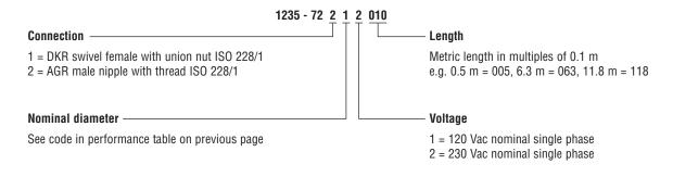
**Example:** 1 m heated hose, 4 mm nominal diameter, 230 V supply voltage, AGR connection **Part Number: 1235-72212010**
