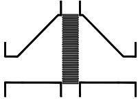
**Bi-directional in-line detonation flame arrester**
