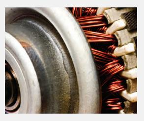
Isopad anti-condensation motor (ACM) heaters have been specifically designed in conjunction with major motor manufacturers to prevent condensation in motor windings which would otherwise lead to sudden or premature failure of the equipment; they are installed around the stator and are popular with manufactures and motor rewind companies alike.
